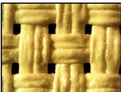
Image 3: Fiberglass Core Fabric Surface (80x)
