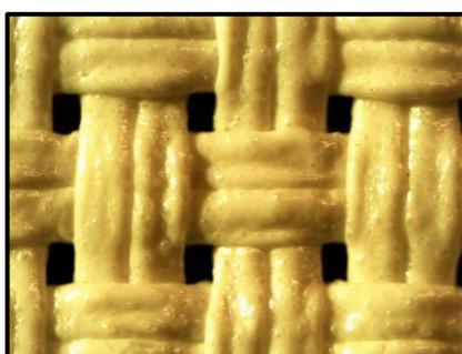
Image 3: Fiberglass Core Fabric Surface (80x)
