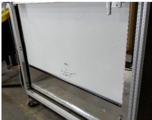
Image 10: Fiberglass Core Fabric in Heatbox
